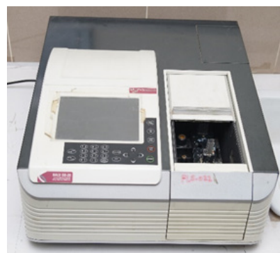
UV-VIS spectrophotometer o Absorbance: -3 to 3 Abs o Transmittance: 0% to 300%
